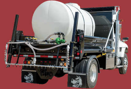
HYDRAULIC ANTI-ICE SYSTEM WITH FLOW METER FOR AUTOMATIC APPLICATION RATE CONTROL
