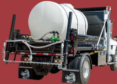
HYDRAULIC ANTI-ICE SYSTEM WITH MANUAL APPLICATION RATE CONTROL
